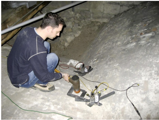
Fig. 13. The hammer operator exciting the pre-determined excitation points with the sledgehammer. Maintaining a relatively consistent excitation level is one of the keys for the success of hammer excitation.
